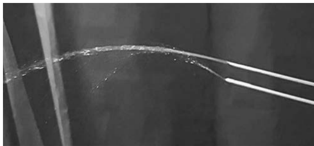
FIGURE 10.8 Comparison of flow characteristics between two needles: Upper needle: 17-gauge STEINER-TAN; lower needle: COOK 17-gauge DL. No linear flow was observed for the COOK 17-gauge DL due to technical characteristics of the needle. (For further information, please see the videos available on YouTube using the key words: Steiner, flushing.)
